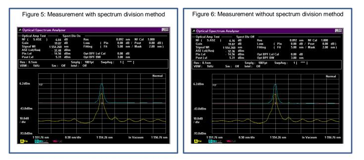
The following example shows the results when an ASE light source (optical noise) is added to a DFB-LD. Figure 7 and 8 show the measurement results with and without the spectrum division method, respectively. Even in this case, the measurement results clearly show that using the spectrum division method suppresses the effect of optical input noise components.
