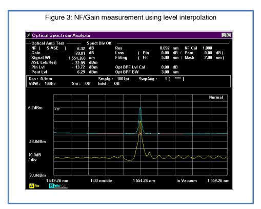
D) Measurements when optical band pass filter (OBPF) inserted at EDFA output
